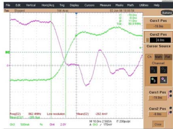
FIGURE 8. Measured current and voltage turn-on switching transient.
